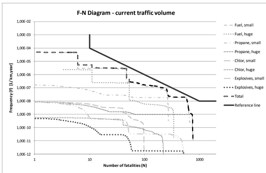
Figure 3: DG risk of Heidkopftunnel (FN curve for Traffic 2010) compared to the German reference line
