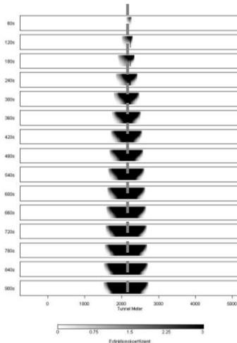
**Figure 17. Smoke propagation along tunnel axis in time steps – zero-flow strategy (scenario 2)**
