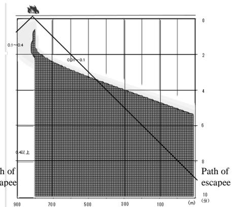
**Figure 8. Smoke density distribution (shut-down control)**
