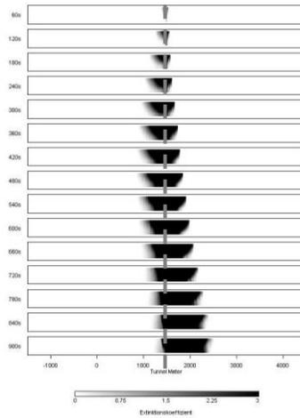
**Figure 16. Smoke propagation along tunnel axis in time steps – shut-down strategy (scenario 1)**
