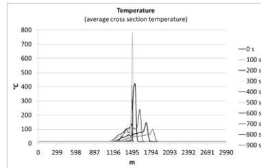
**Figure 14. Average cross section temperature – shut-down strategy**
