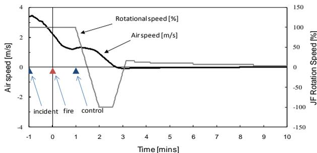
**Figure 1. Rapid achievement of zero-flow by automatic control**
