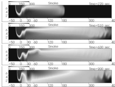
**Figure 3. Predicted smoke density distribution at successive instants**
