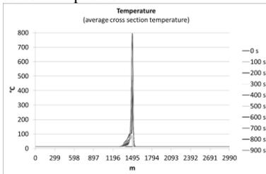
**Figure 13. Average cross section temperature - zero-flow strategy**
