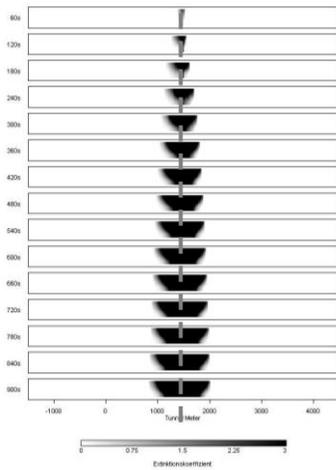
**Figure 15. Smoke propagation along tunnel axis in time steps- zero-flow strategy (scenario 1)**
