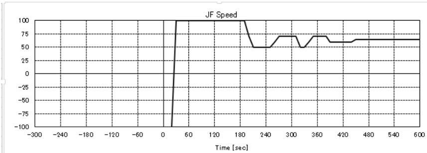
**Figure 6. Air flow velocity and jet-fan speed in the 1D simulation (zero-flow control strategy)**
