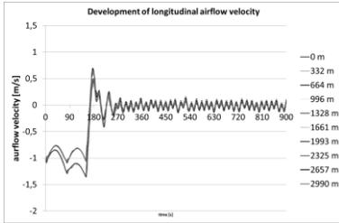
**Figure 11. Development of longitudinal airflow velocity – zero-flow strategy**
