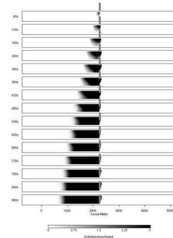
**Figure 18. Smoke propagation along tunnel axis in time steps – shut-down strategy (scenario 2)**
