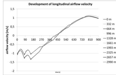
**Figure 12. Development of longitudinal airflow velocity – shut-down strategy**
