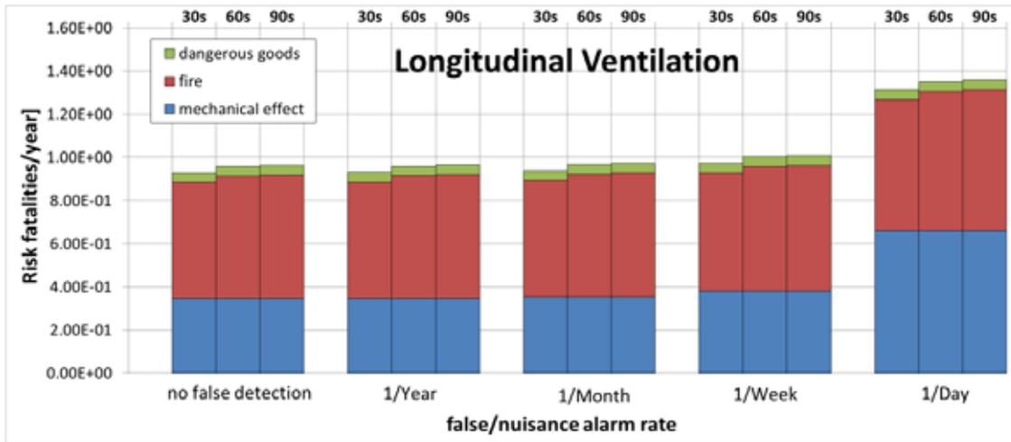
**Figure 6:** Risk (fire risk + collision risk) dependencies on false/nuisance alarm rate and fire detection time for standard-flow ventilation control
