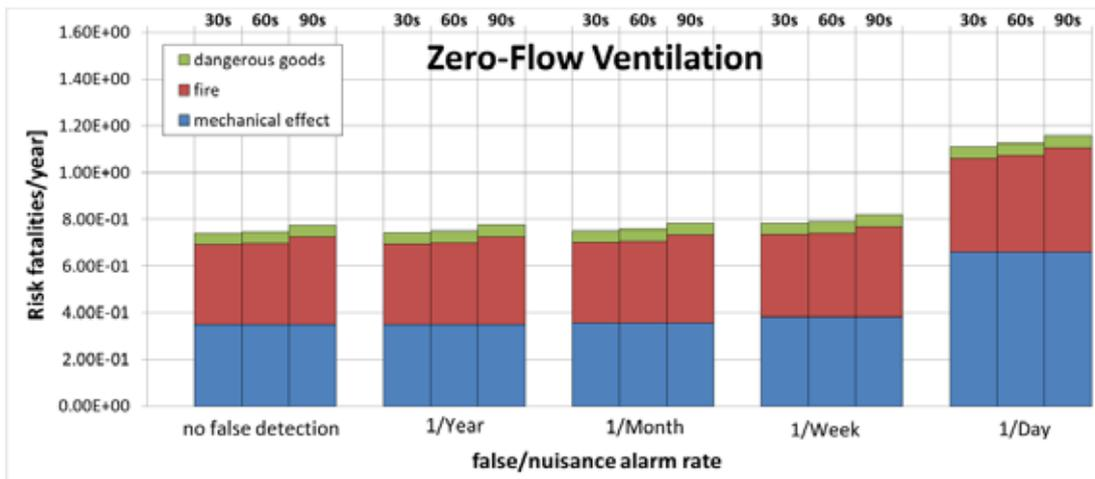
**Figure 7:** Risk (fire risk + collision risk) dependencies on false alarm rate and fire detection time for zero-flow ventilation control
