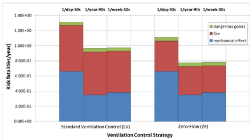
**Figure 8:** Comparison of selected false alarm rates and fire detection time combinations
