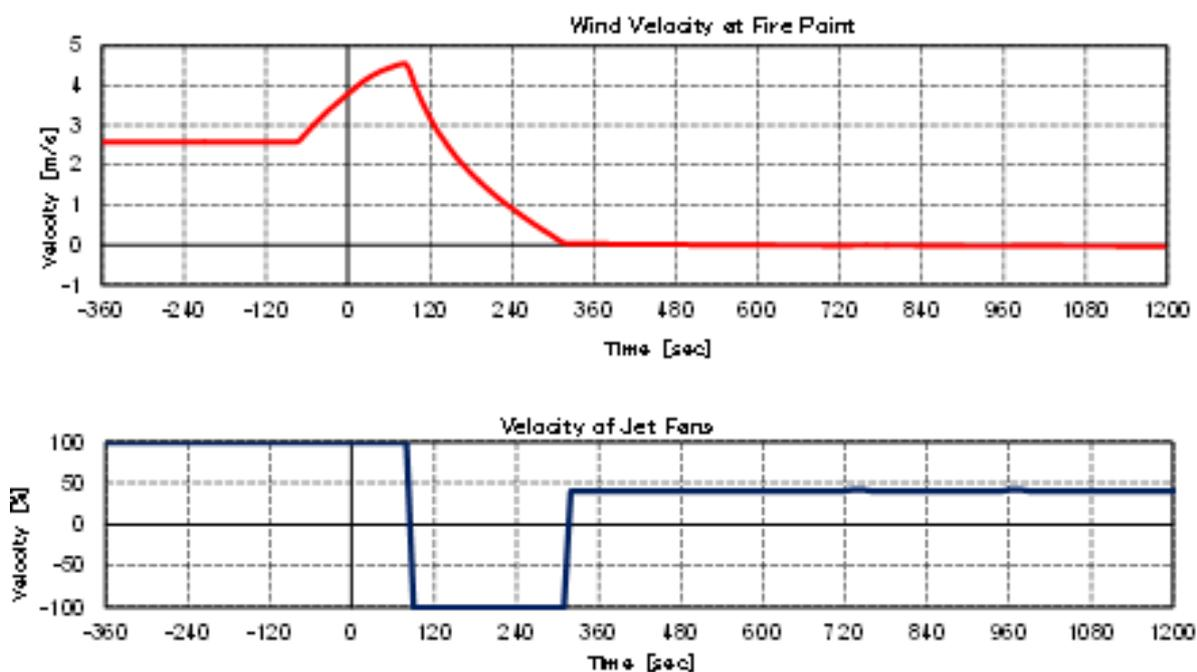
**Figure 2:** Air-flow velocity and output of jet-fans: 90s delay in fire detection
