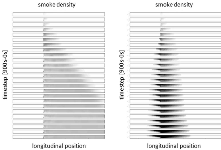
**Figure 6: Comparison of smoke propagation for critical-velocity ventilation (left) and zero-flow ventilation (right) – 5MW**
