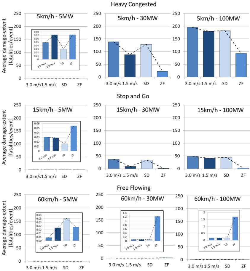
**Figure 8: Collected results for damage-extent [fatalities/event] in the event of a tunnel fire. To facilitate comparisons, a common scale (0-250) has been chosen for the average damage-extent values for all scenarios. In addition, for scenarios with very low damage-extent values, figures with a smaller scale have been included**
