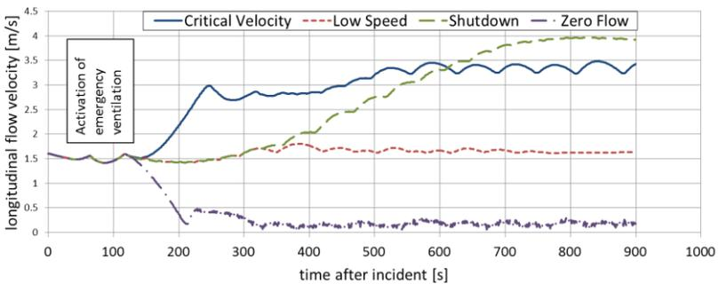
**Figure 5: Development of longitudinal airflow velocity for a 100MW fire**
