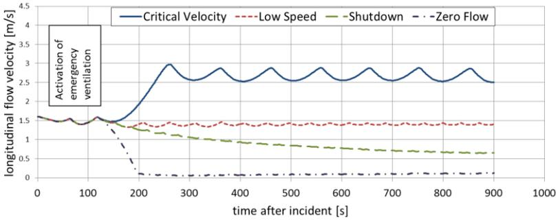
**Figure 4: Development of longitudinal airflow velocity for a 5MW fire**
