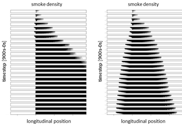
**Figure 7: Comparison of smoke propagation for critical-velocity ventilation (left) and zero-flow ventilation (right) – 100MW**
