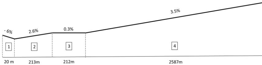
Figure 3: Longitudinal profile of the model tunnel
