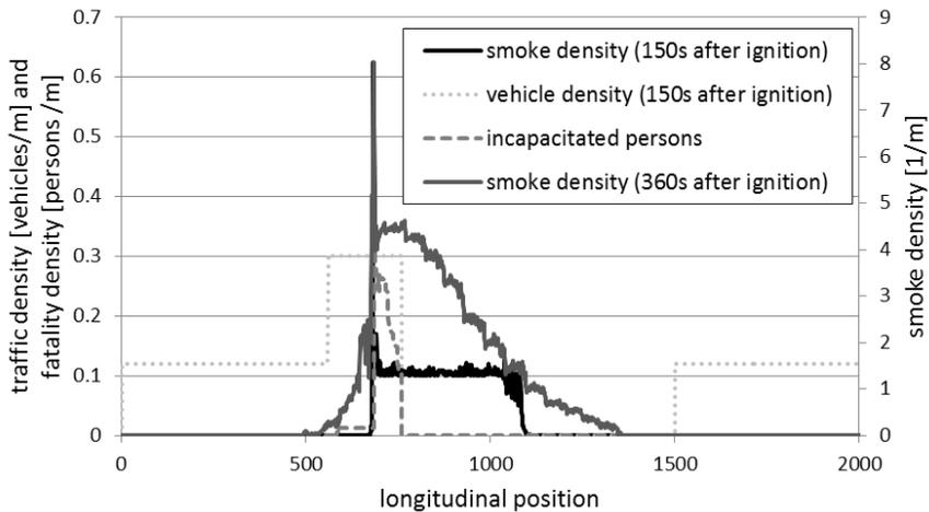
**Figure 2: Smoke density- (solid line), vehicle density- (dotted line) and fatality density distribution (dashed line) for one exemplary fire scenario (30 MW/stop and go/zero flow ventilation)**
